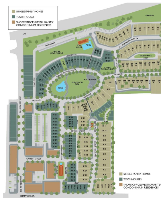
Figure 28: Glenwood Park site design with small, shared parking lot for multi-family units
